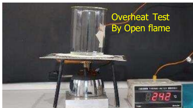
Heat Test Iwaki CTE33 Beaker product without liquid with burner up to 240 °C. Test Result: PASS
