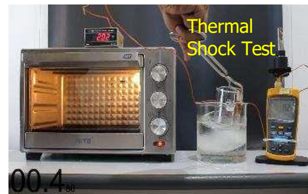
Thermal Shock Test of Iwaki CTE33 Beaker Glass with \Delta T \geq 190 °C transfer time 4 seconds. Test Result: PASS
