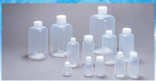
NAFLON™ PFA CHEMICAL WARES are the containers made from PFA fluorocarbon resin and made by the blow molding method. They have the exceptional chemical resistance, and little elution of impurities for almost all kinds of fluids. What is more, they have higher mechanical strength compared with the glass wares and are unbreakable even if dropped.
